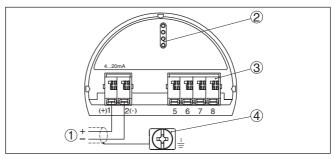
Fig. 36: Electronics and connection compartment - single chamber housing
