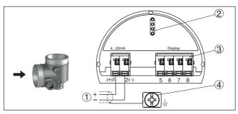
Fig. 29: Connection compartment - double chamber housing
