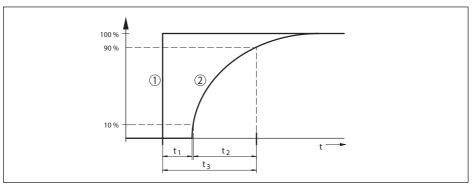
Fig. 49: Behaviour in case of sudden change of the process variable. t,: dead time; t,: rise time; t,: jump response time
