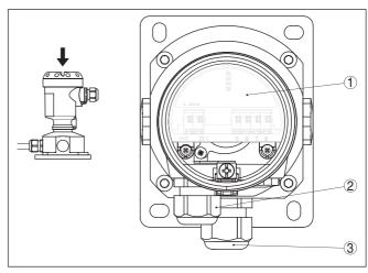
Fig. 34: Electronics and connection compartment
