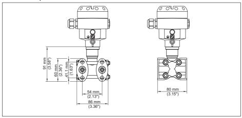
Fig. 52: DPT-20, ventilation on process axis
