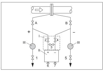
Fig. 46: Preferred measurement setup for liquids
