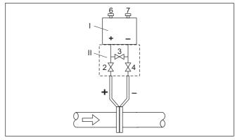
Fig. 45: Prefered measurement setup for gases, connection via 3-fold valve block, flanging on both sides
