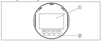
Fig. 40: Display and adjustment elements
