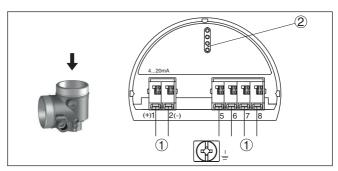
Fig. 28: Electronics compartment - double chamber housing
