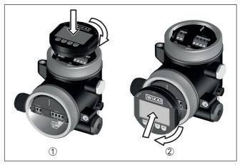
Fig. 39: Installing the display and adjustment module in the double chamber housing
