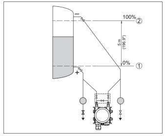
Fig. 41: Parameter adjustment example "Min./max. adjustment, level measurement"
