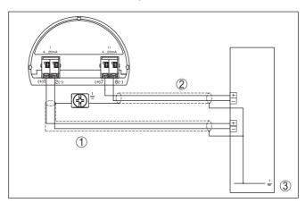
Fig. 37: Connection example DPT-20 additional current output
