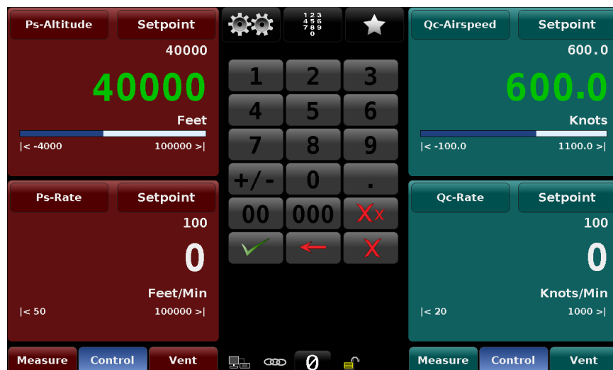
Figure 6.2.2 - Altitude and Airspeed Reading (shown in green)
