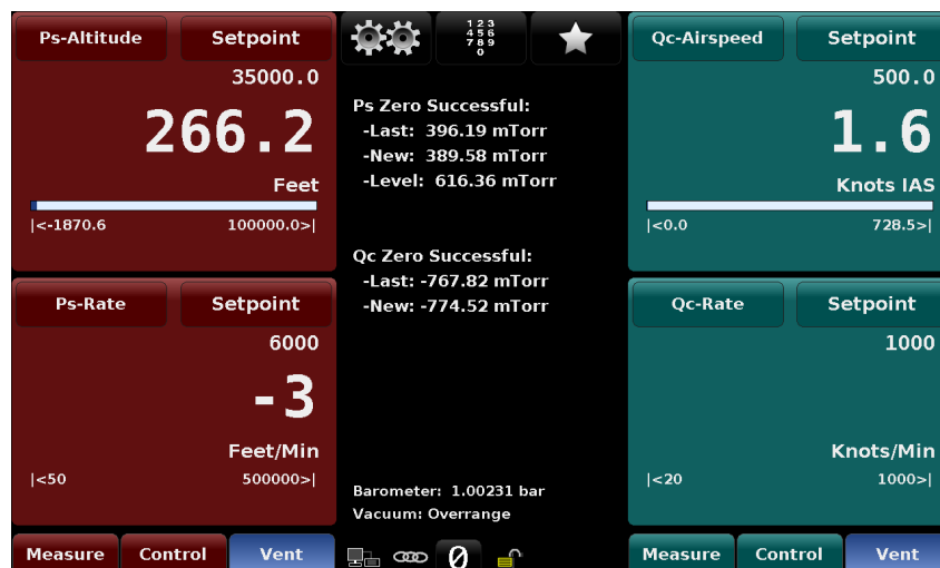
Figure 6.2.15c - Zero Sequence, 120 second delay
