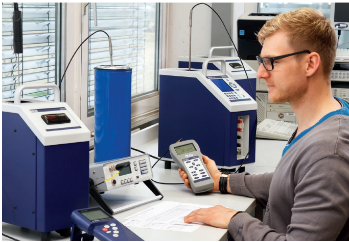
Comparative calibration in the Wika calibration laboratory
